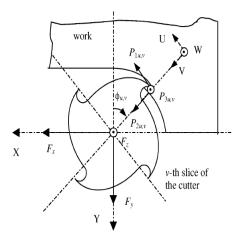
Fig. 4. Coordinate systems for the vth slice of the milling cutter.
