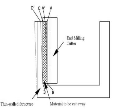
Fig. 1.Machining sketch of the typical thin-walled structure.
