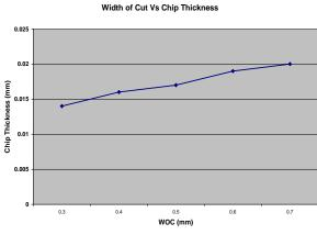
Fig. 10. Effect of width of cut on chip thickness
