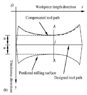
Fig. 15 2-D view of Error compensation profilein section A–A at cutting position *j*.
