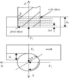
Fig. 2.Model for End milling Process
