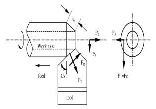
Fig. 3.Model for simple oblique cutting.
