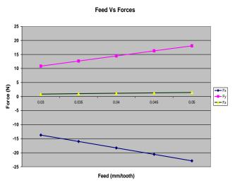
Fig. 7. Effect of feed on cutting forces
